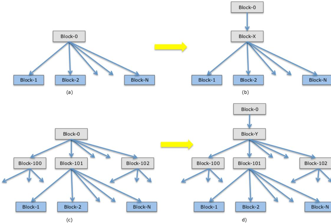
(a) and (b) show htree growing from 1-level to 2-level. (c) and (d) illustrate htree growing from N-level to (N+1) level. A new DX-block is added as the only child of DX-block 0 and obtains children of DX-block 0.
