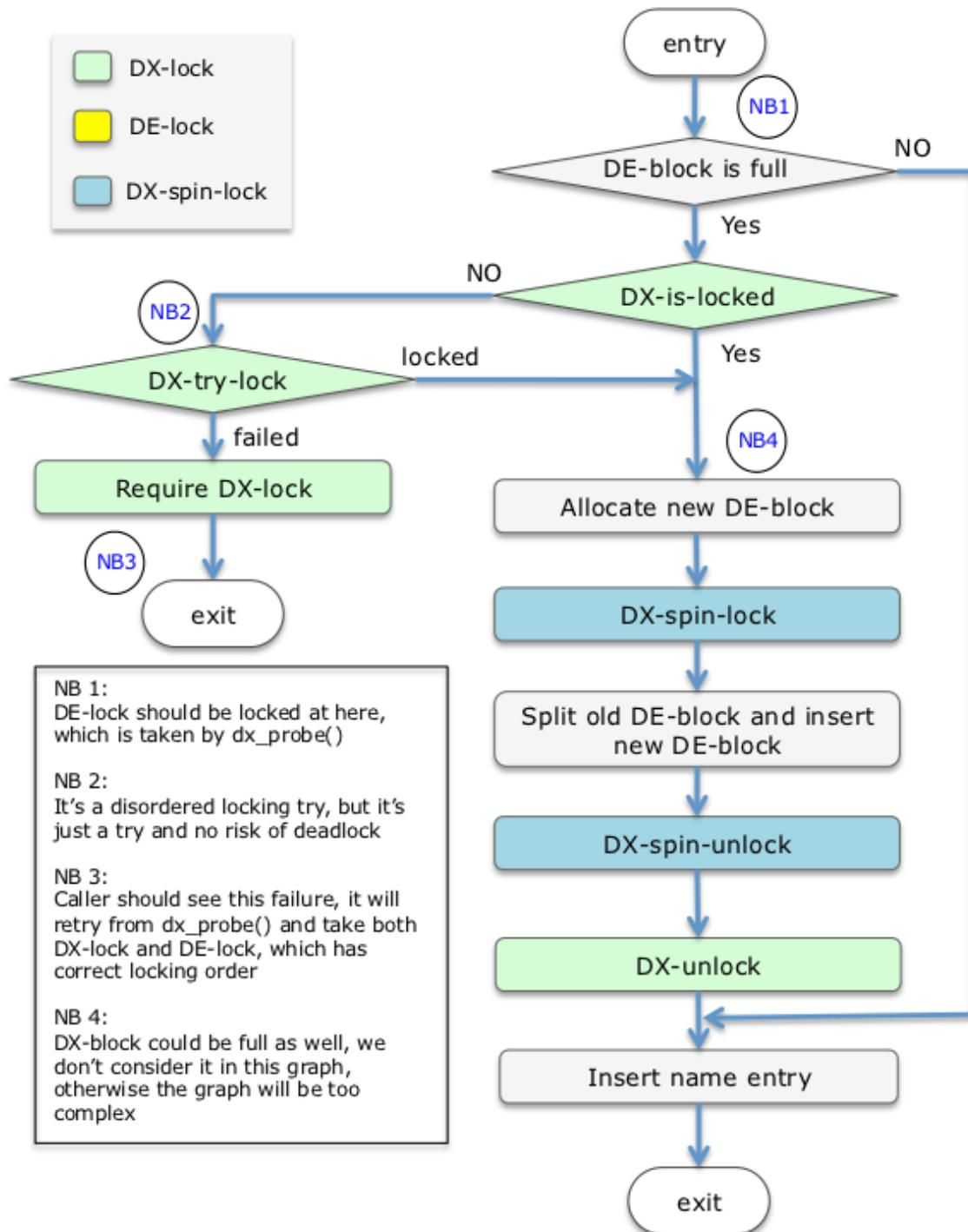
If the DX-block is full or the tree is full and needs to grow, we just need to lock the whole htree with EX mode and repeat the process of `dx_probe()` and `dx_add_entry()`.
