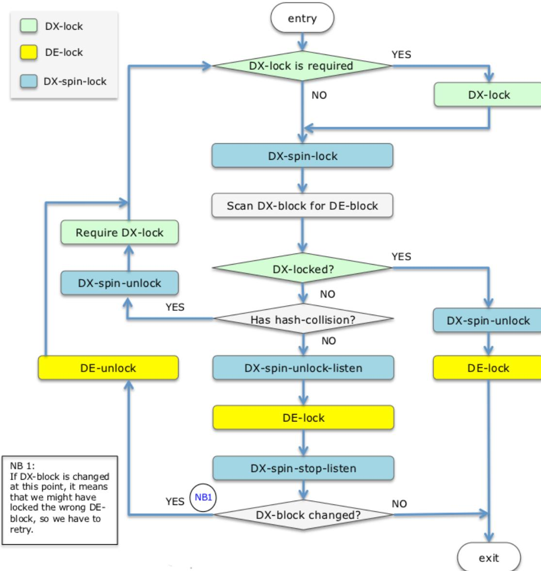
The figure above illustrates the logic using child-locks of htree-lock to protect the process of `dx_probe()`. The method is:
