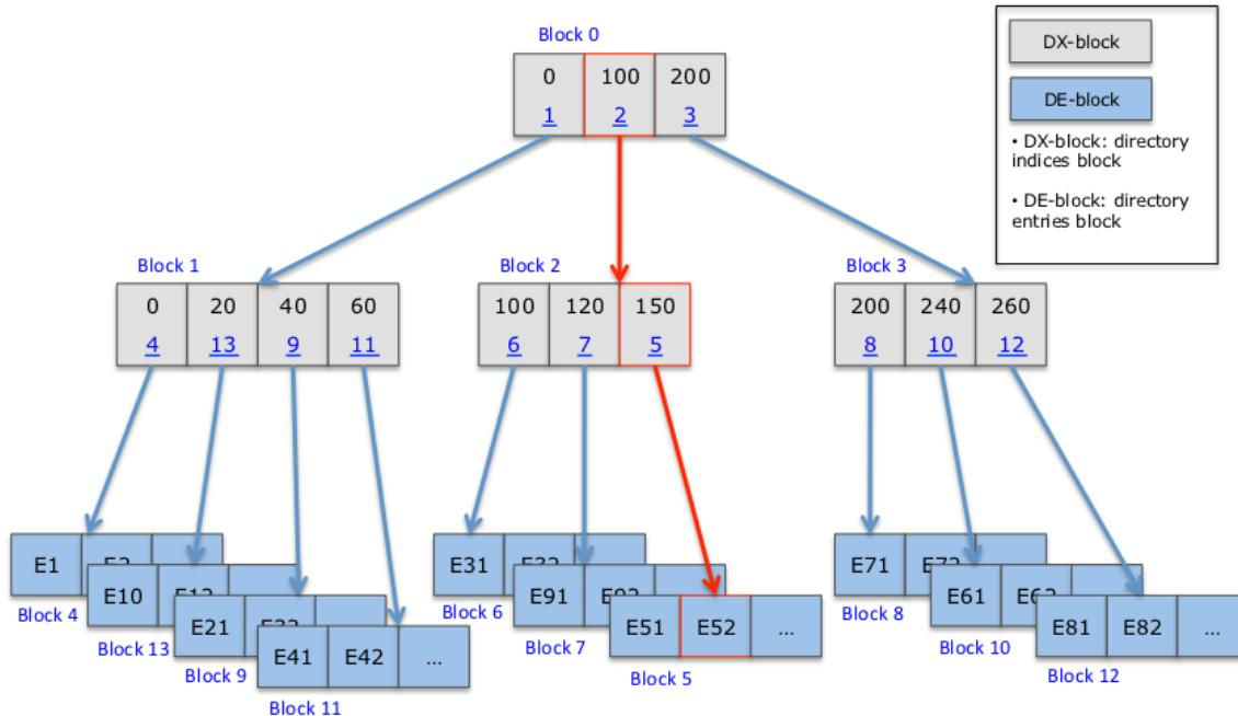
A tree node path for a name entry. The red line in Graph-1 is htree path for name E52.
