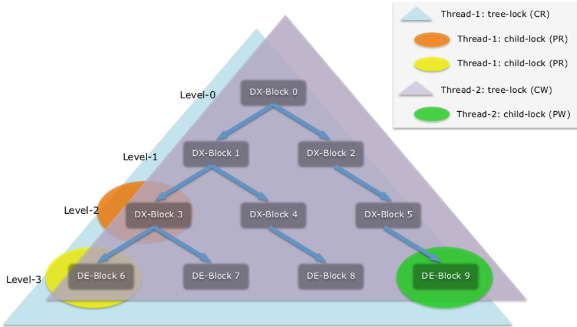
Two types of locking operation are available: tree-lock and child-lock. Graph-2 shows how they are used to protect htree directory.
