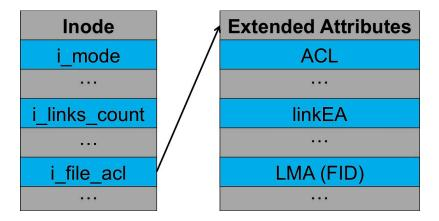
During a file-level backup, all the extended attributes are archived. When a file level backup archive is restored, new inodes are created, and the extended attributes are restored. At this point, records in the OI table (which is stored in the filesystem as a regular file) are incorrect as new inode numbers are allocated to the restored files.
