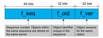
A FID is recorded in the extended attribute (called the Lustre Metadata Attribute, LMA) of an inode to allow mapping from the inode to the FID number, and for redundancy. The figure below illustrates the FID as a Lustre Metadata Attribute. In order to allow inode lookups by FID number, a table of FID-to-inode entries is maintained. This table is called the OI Table.
